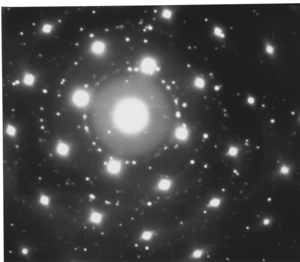
Figure 25 Diffraction pattern of peak aged Cu-0.7%Cr-2.0%Fe alloy. Additional reflections and semi-continuous rings due to incoherent precipitates are visible. Beam direction B = [1, 0, 0] .
